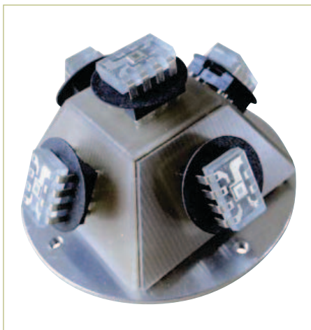
Figure 1. The five measuring sensors assembled at fixed angles.
