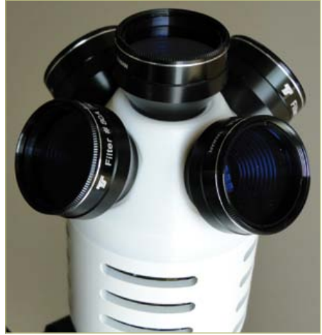
Figure 3. Construction of the sensor with the filters.
